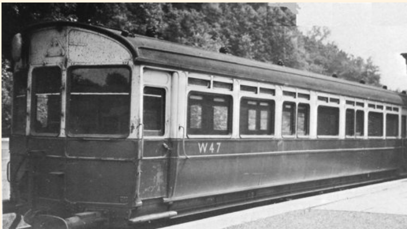
An auto trailer at Tetbury station waits for the driver to move from the engine behind it and set off back to Kemble. This one was one of Lot 1108 built at Swindon in early 1906.
