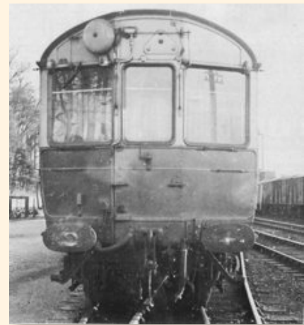
Front view of an auto trailer. As well as being able to blow the whistle from his cab the driver could also stamp on a pedal to sound a gong to warn of the train's approach.
